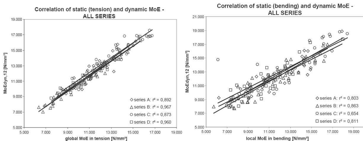
Figure 4. Relations of static and dynamic MoE for tension (le) and bending (ri)
