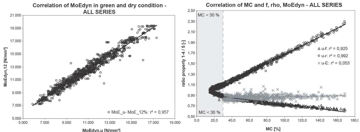
**Figure 1. Correlation of dynamic modulus of elasticity in green and dry condition (le); Correlation of moisture content and the ratios of dynamic properties and density (ri)**
