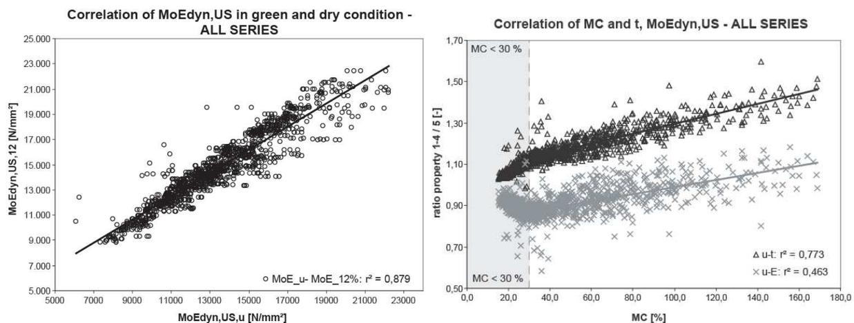
**Figure 2. Correlation of dynamic modulus of elasticity (US) in green and dry condition (le); Correlation of moisture content and the ratios of dynamic properties (ri)**
