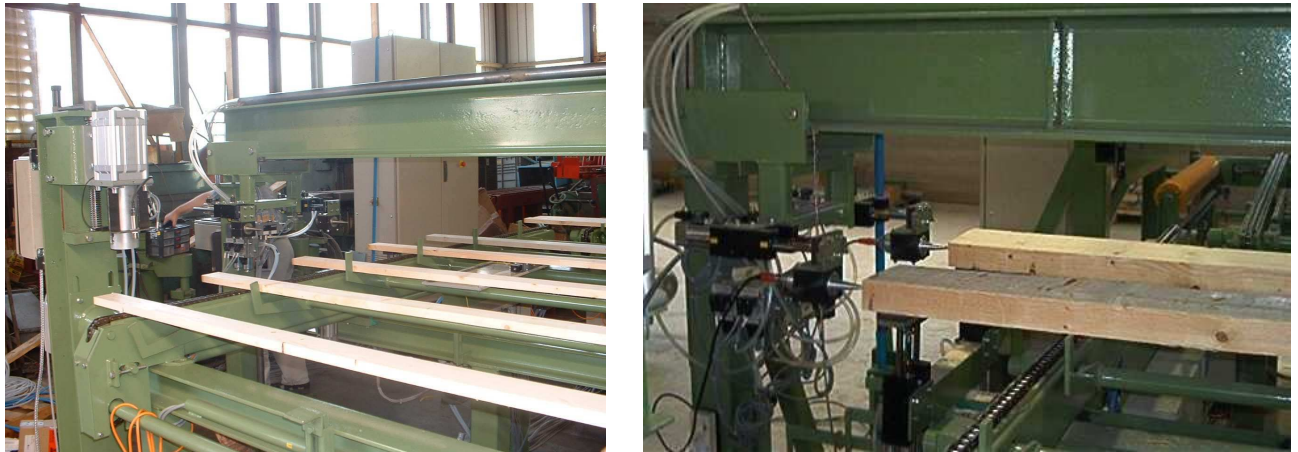
Figure 5: Ultrasonic module composed here by two pairs of transducers. Triomatic Ecolam, Belgium. More pairs could be added in order to increase the process if needed.
