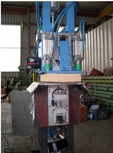
Figure 6: Density and moisture content measurement module. A jaw composed by two load sensors on which a pair of pins is screwed measures the wood local density from above and from under the plank. The moisture content is simultaneous measured once the pins are in the wood. Triomatic, Ecolam, Belgium.
