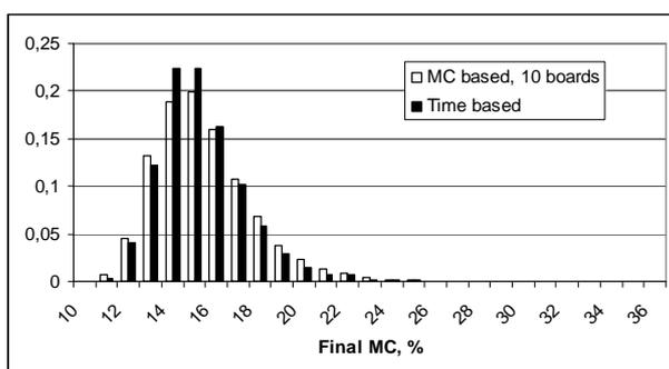
Figure 7. Final MC distributions for a MC based drying schedule with 10 control boards and for a time based schedule. Target final MC is 16 %.
