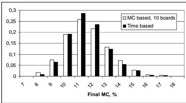
Figure 8. Final MC distributions for a MC based drying schedule with 10 control boards and for a time based schedule. Target final MC is 12 %.
