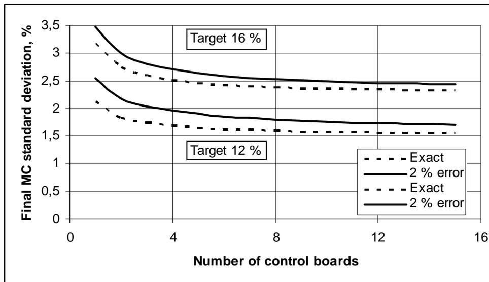
Figure 6. Influence of control board MC measurement error on the final MC standard deviation.
