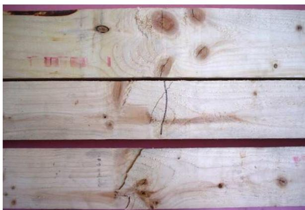
Figure 7. Machine grader rejects with severe cross grain.
