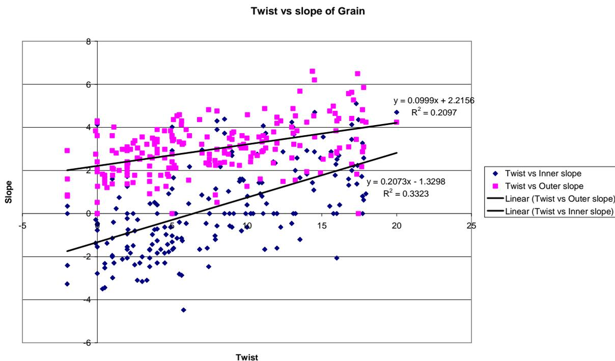
Figure 1. Twist (mm) plotted against slope of grain (deg)
