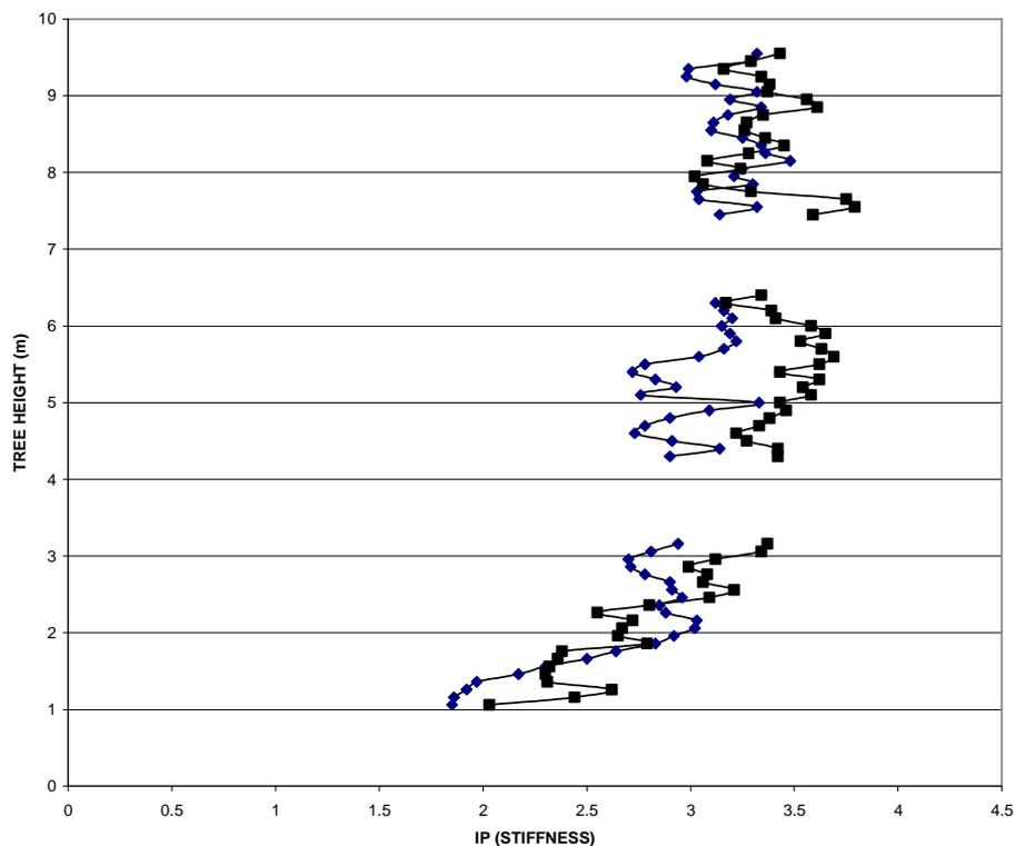
**Figure 4. Batten stiffness profiles showing low stiffness at the base of trees.**
