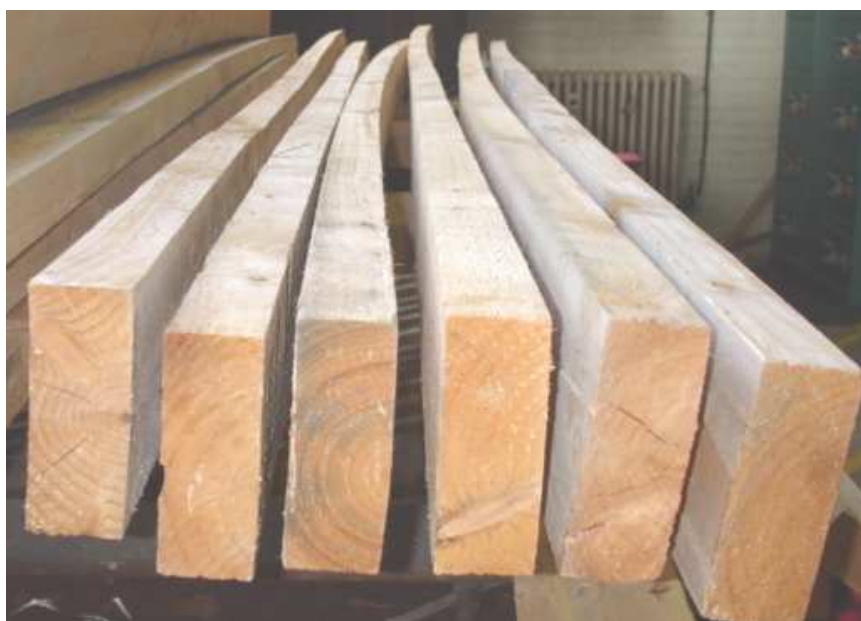
Figure 2. Bow of timber dried unrestrained, caused by juvenile wood and compression wood.
