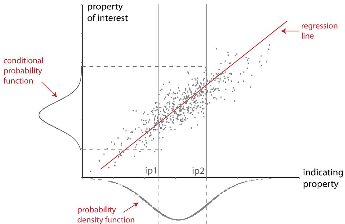
**Figure 2:** *Alternative approach for the control of grading machine settings, based on the regression analysis. Based on the regression analysis and the probability density function of the indicating property, first an conditional probability function and out of this an predictive distribution function of the property of interest can be assessed.*
