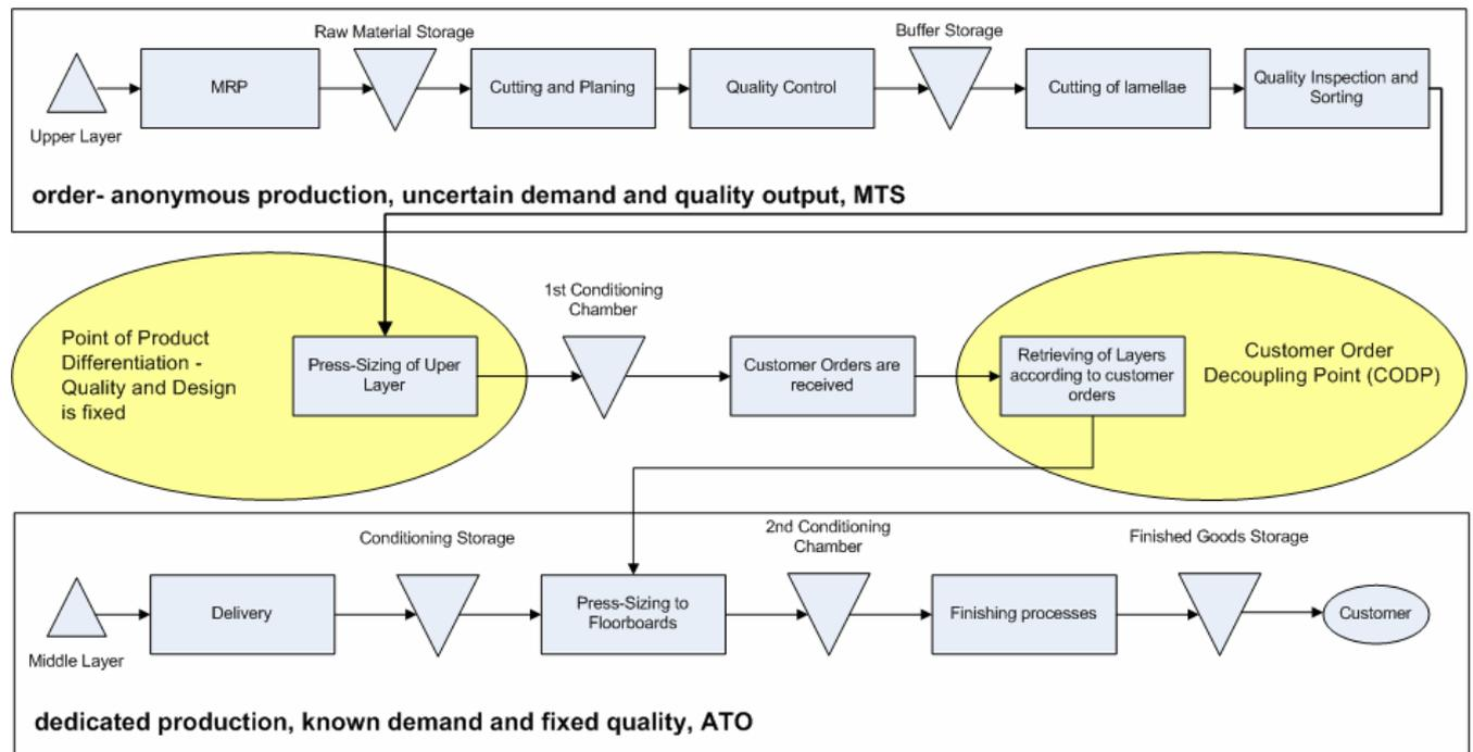
Figure 1. Production Processes including PPD and CODP
