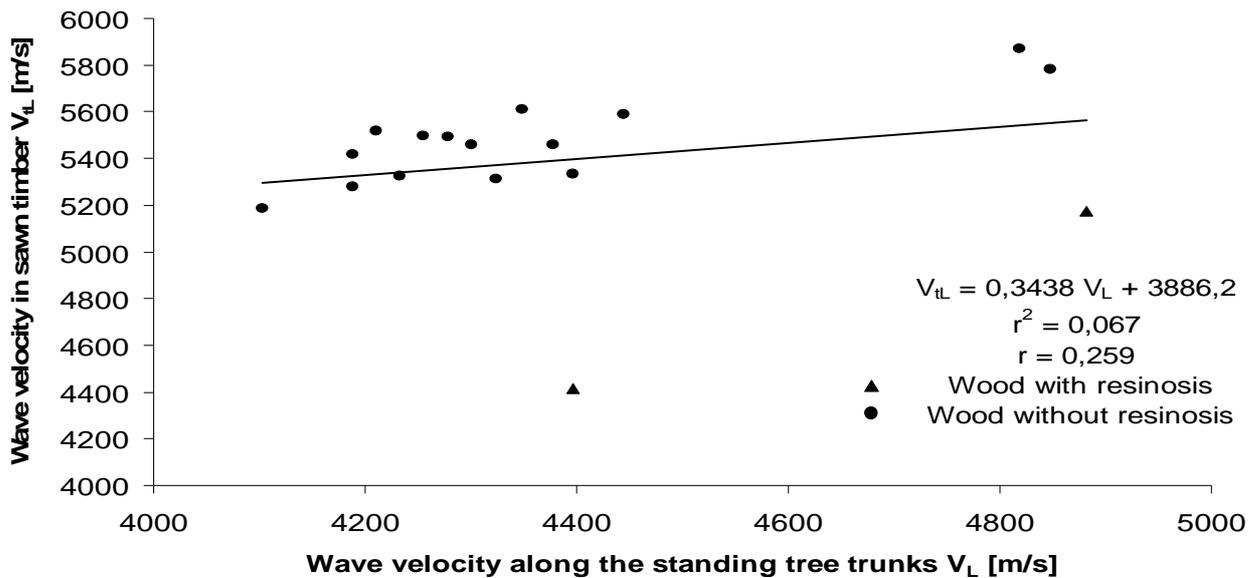
Figure 2. Correlation of ultrasonic wave velocity in standing tree trunks and sawn timber – including wood with resinosis.
