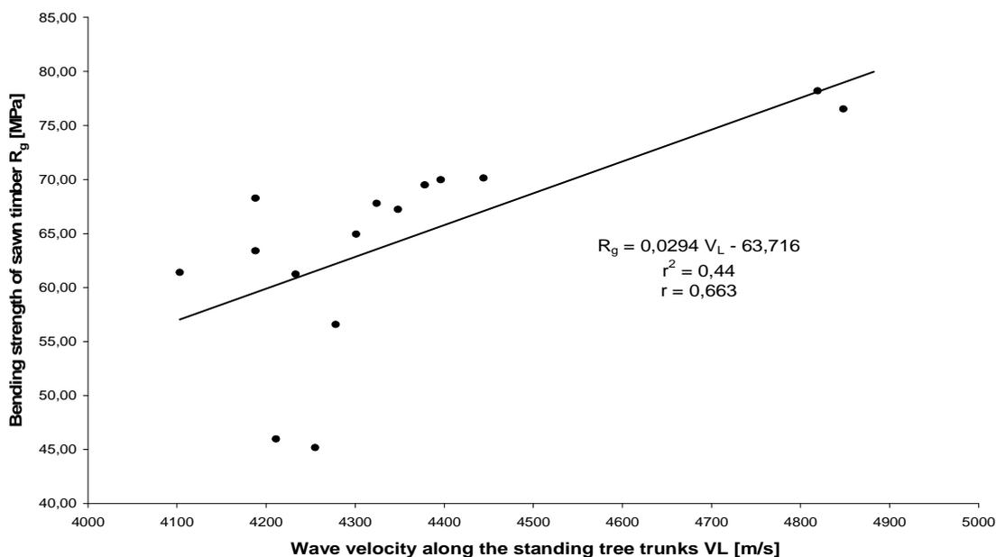
Figure 4. Correlation of bending strength of sawn timber and ultrasonic velocity along standing tree trunks.
