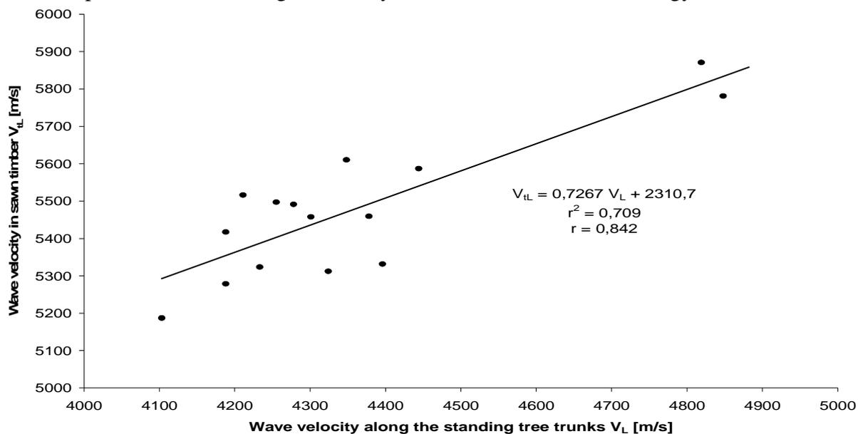
**Figure 1. Correlation of ultrasonic wave velocity in standing tree trunks and sawn timber.**
