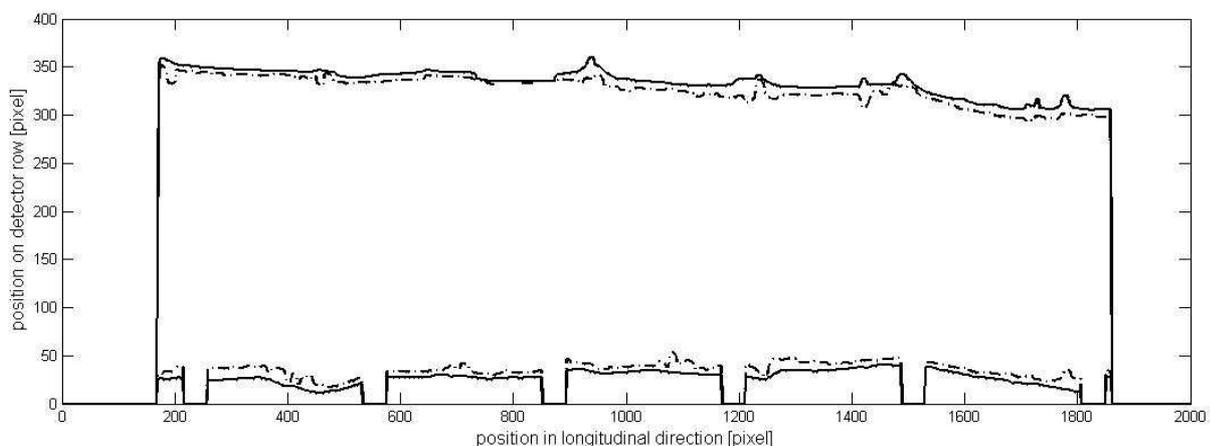
Figure 2. Shape of the log (continuous line) and of the recognized solid wood (dashed line); missing parts in the downer lines are caused by the conveyor where neither the outer shape nor the shape of solid wood can be detected
