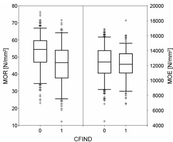
**Figure 1. Effect of the presence of CF (CFIND) on MOR and MOE. Box plots for sub-samples without and with CF. (Boxes show the median together with 25th and 75th percentiles, whiskers extend to 5th and 95th percentiles.)**
