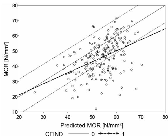
**Figure 2. Relationship between predicted and observed MOR for the beams with CF. (The thin solid and dotted lines are the linear regression line and the 90% confidence bands for individual predicted values respectively of the regression model built on the sub-sample of the beams without CF. The thick dotted line is the linear regression line for the beams with CF.)**
