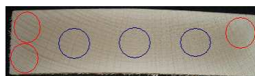
Positions of color measurement along the edge (red) and in the core (blue) (cross section of specimen)
