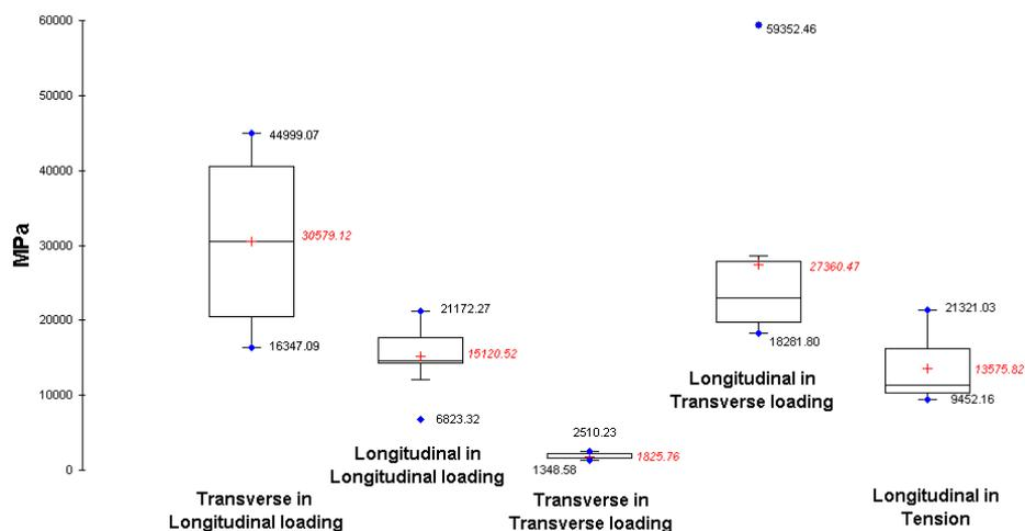
Figure 3: Material properties of barrel oak
