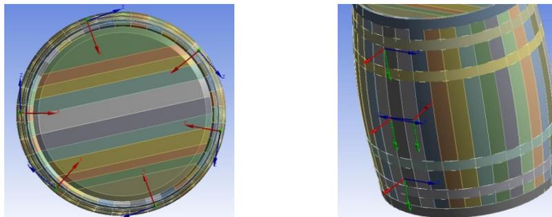
Figure 2: FEA displacement probes about the barrel bilge
