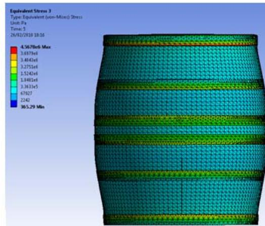
Figure 9: FEA image of stress distribution for optimised 1:2.5
