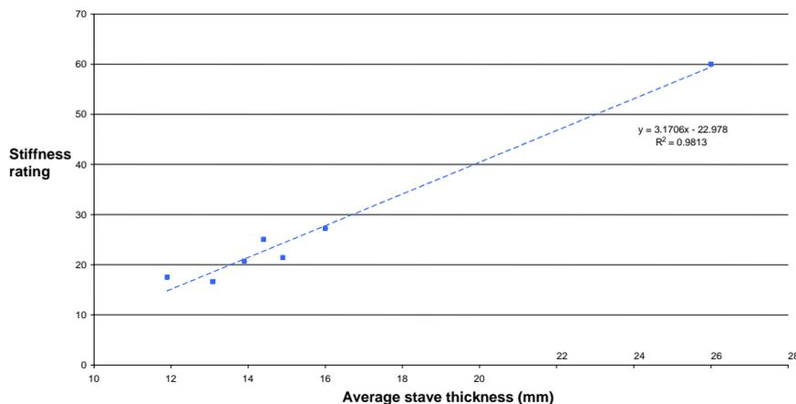
Figure 4 – Stiffness rating comparison of thinned barrels
