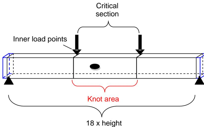
Figure 2: Knot area between the inner load points at bending test
