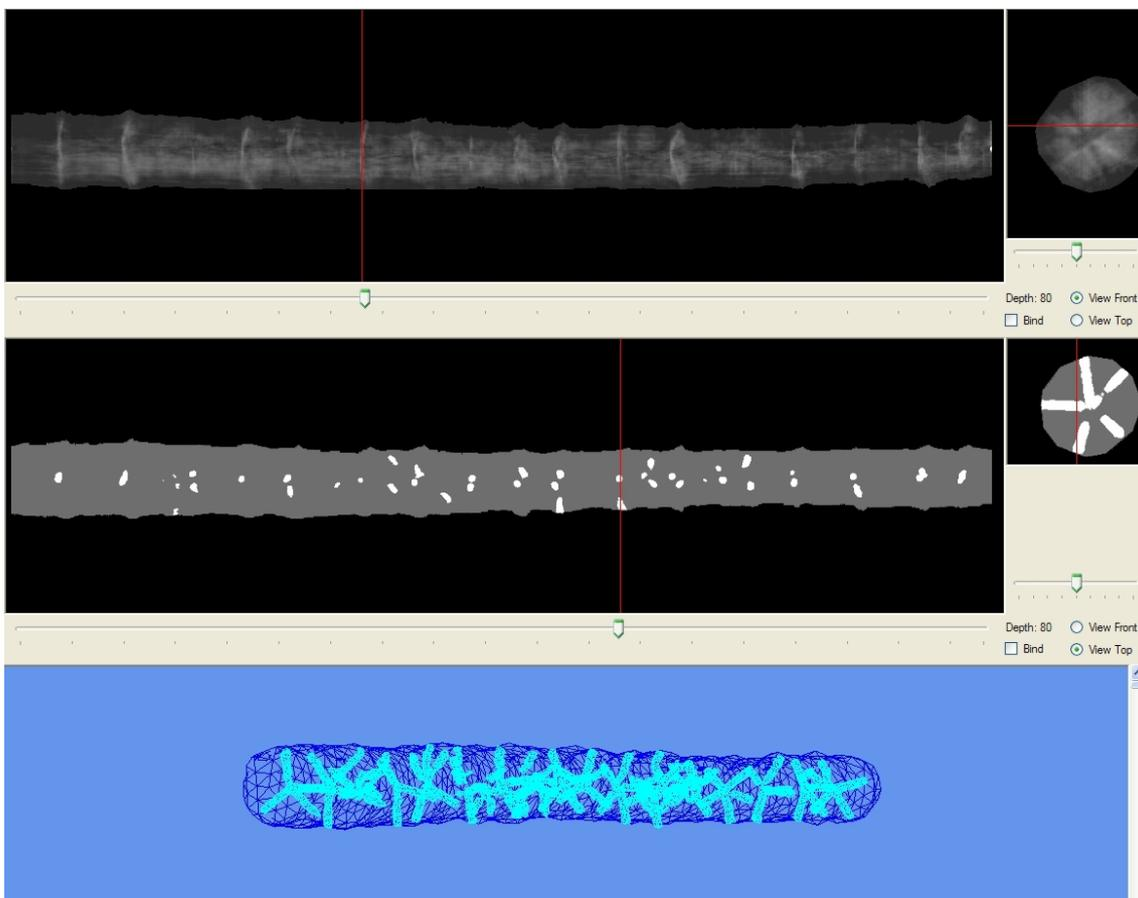
Figure 5: 2D X-ray picture of a log
