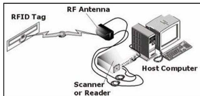
Figure 1. The basic elements of an RFID system
