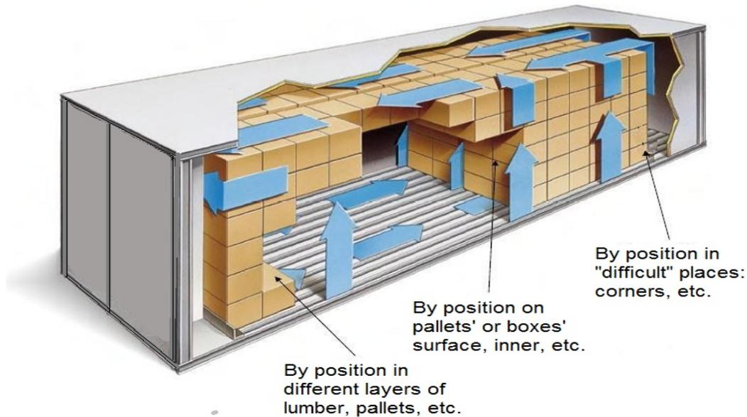
Figure 4. RFIDs can be placed anywhere in a dry kiln or heat-treatment chamber, in order to record temperatures.
