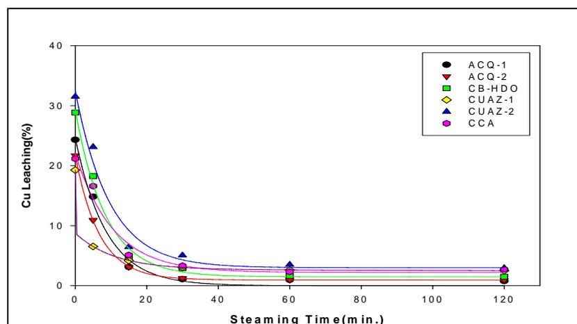
Figure 6. Effect of post steaming treatment on copper fixation in different copper amine preservatives treated radiate pine sapwood.
