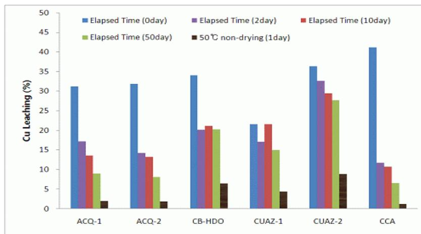
Figure 5. Cu leaching (%) from different preservatives treated radiate pine sapwood at 20 °C with drying, compared to 50 °C without drying conditions.
