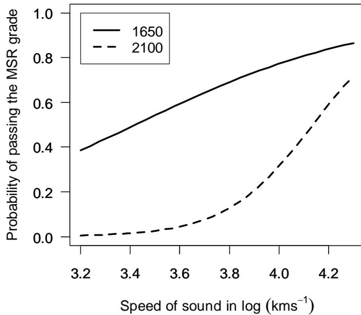
Figure 3: Probability of obtaining a 2'x'4 piece of the '1650' and '2100' MSR grades as a function of the speed of sound in the log (white spruce only)
