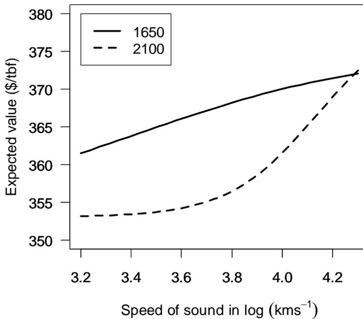
Figure 4: Expected value of one thousand board feet (tbf) of lumber as a function of the speed of sound in the log (white spruce only)
