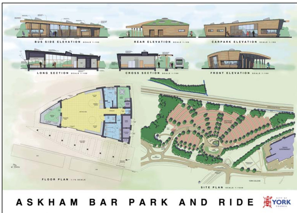
Figure 14 – One of three terminals which would ideally be constructed with a timber sub-structure and super-structure
