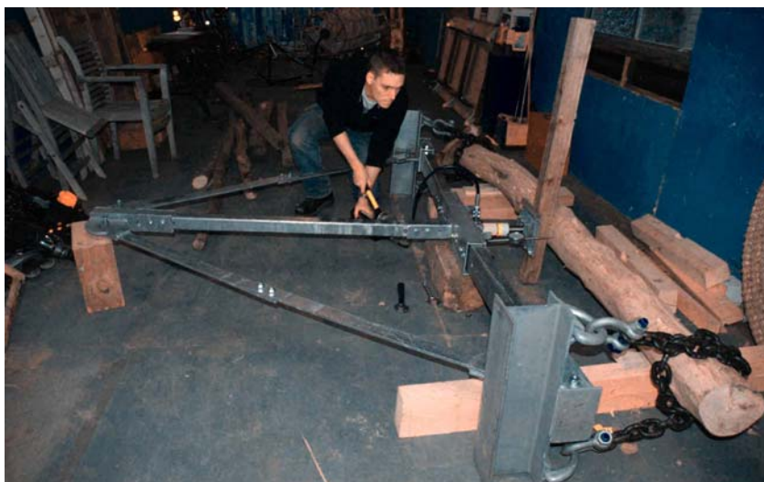
Figure 5 Portable test rig capable of 10Tonnes point load for checking the ultimate strength or the stiffness of beams between 2 to 6m long. It would not be considered practical or safe to determine the capacity of this uncut and curved sycamore log by using just visual grading and currently available data.
