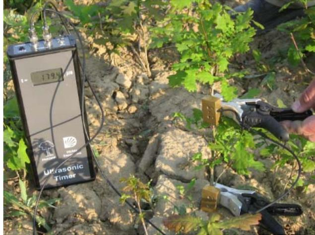
Figure 1. The seedling tester device is in a nursery. Manufactured by FAKOPP Bt. Hungary, [www.fakopp.com](http://www.fakopp.com)
