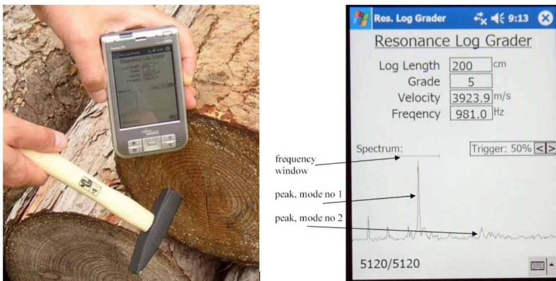
Figure 4. The log grader in a log yard. And the PDA screenshot.
