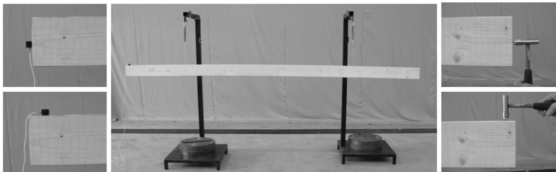
Figure 1: Test setup for assessment of dynamic MOE.
