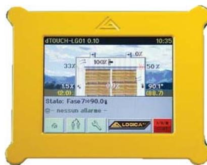
Figure 3: Touch screen of the control unit: main page
