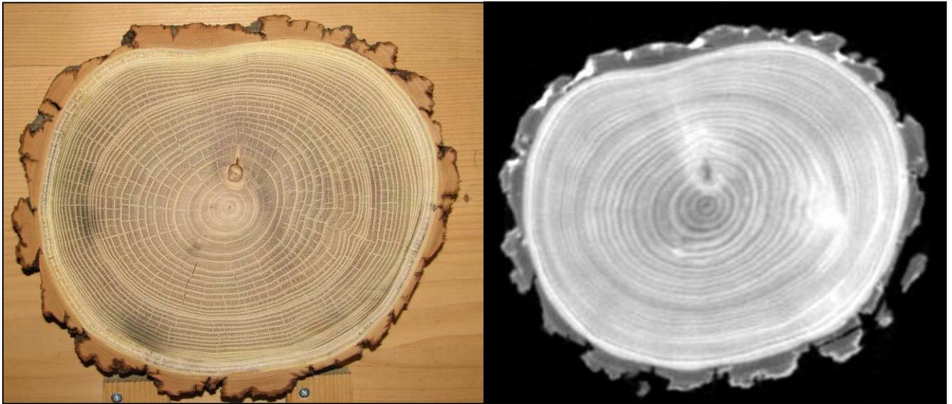
Figure 1: *Robinia* stem disc (left) and CT reconstruction slice (right)
