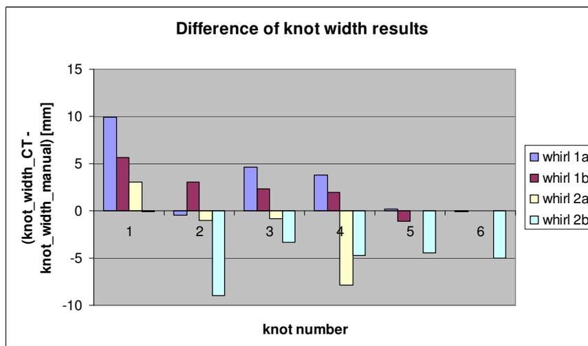
Figure 8: Difference between manual and CT measurement of the knot width
