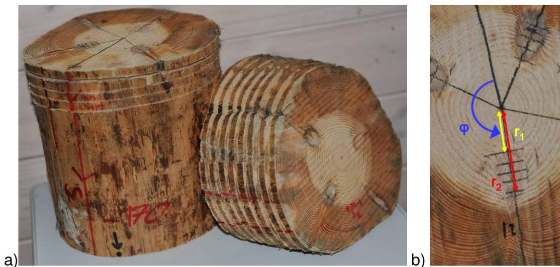
Figure 3: a) Discs from one whirl used for manual measurements; b) Manual measurements for one knot on one disc
