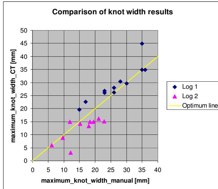
Figure 7: Results of knot width measurements
