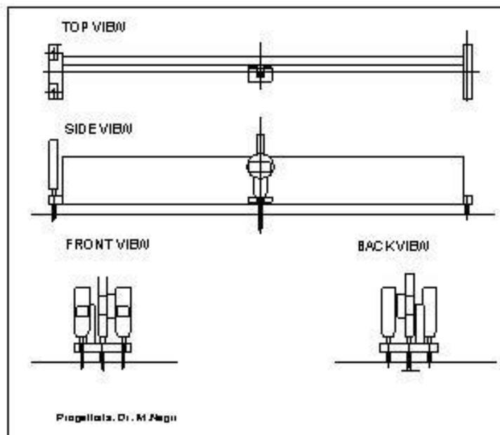
Figure 1 - The reference bar instrumented with gauges
