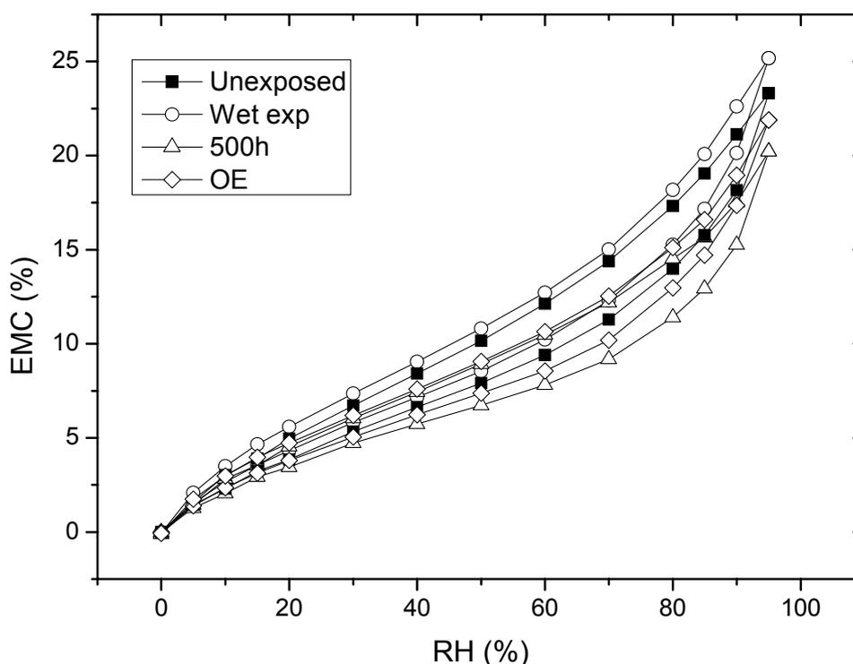
Figure 2: Sorption Isotherms for latewood samples post exposure
