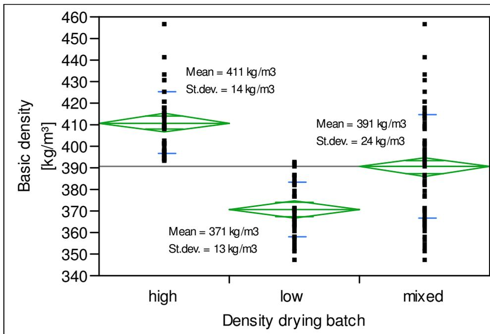
Figure 1: The distribution, mean and standard deviation of the basic density in the drying batches
