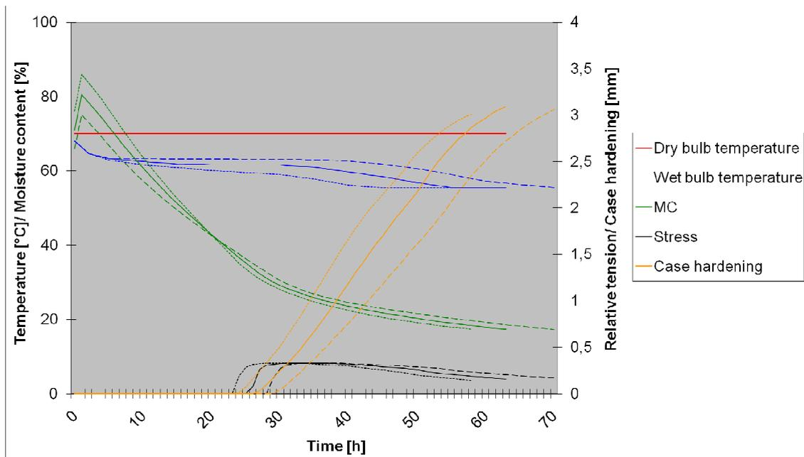
Figure 2: Drying schedule for the three drying batches with simulated development in moisture content, stress, and case hardening according to Torksim (Tråtek 2001) (— mixed density batch, --- high density batch, ··· low density batch)
