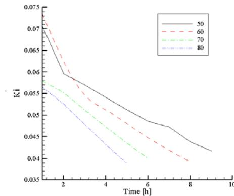
Figure 2: Hygrometric criterion variation in time for RH=40% and different dry-bulb temperatures
