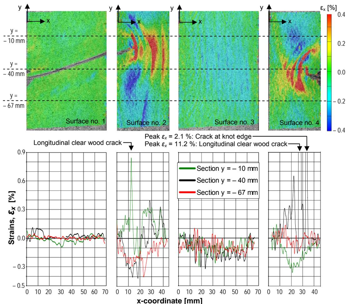
Figure 6: Lateral surface strains ( $\epsilon_x$ ) for maximum load 30 kN, recorded for Load tests no. A1-A4. Top row: Contour plots. Bottom row: Section diagrams for the sections (dashed lines) shown in the top row.
