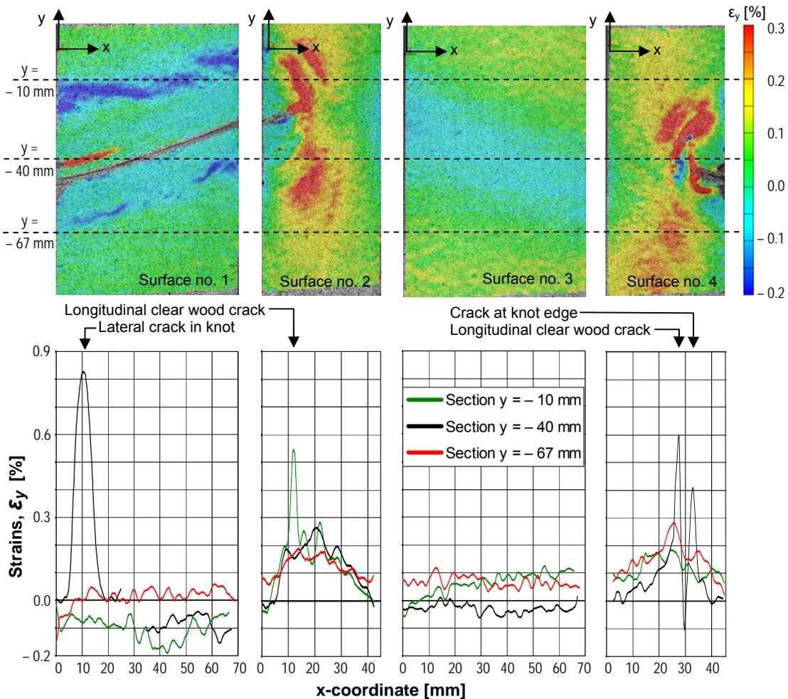
Figure 5: Longitudinal surface strains ( $\epsilon_y$ ) for maximum load 30 kN, recorded for Load tests no. A1-A4. Top row: Contour plots. Bottom row: Section diagrams for the sections (dashed lines) shown in the top row.
