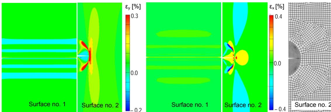
Figure 7: Results from FE simulation: Longitudinal strains (left), Lateral strains (middle) and FE mesh (right).
