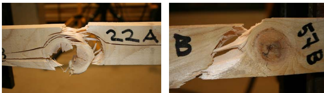
Figure 13: Fractures in two of the weakest split boards in the sample.
