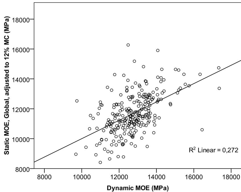
Fig. 2: A scatter plot and a linear regression line showing the relationship between the ultrasound velocity-based dynamic MOE and static bending MOE of glulam beams made of Scots pine or Norway spruce.
