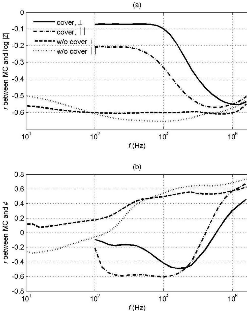
Figure 4.(a) The correlation coefficient  $r$  between MC and  $\log |Z|$  for heartwood specimens. (b) The correlation coefficient  $r$  between MC and  $\phi$  for heartwood specimens.  $N = 37 - 42$ , and correlations are significant at 5 % level around  $r = 0.35$ .
