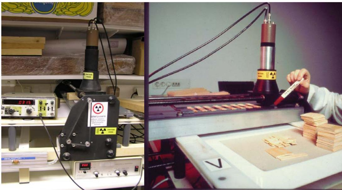
Figure 3. Gamma ray measurement of wood and veneer sheet specimens.
