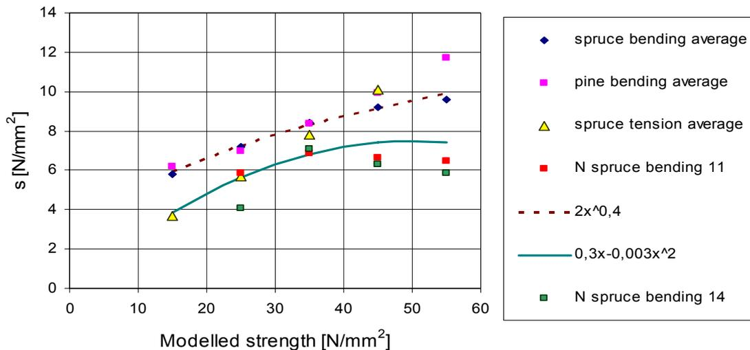
Figure 2: Average standard deviation of strength of European timber of 10 N/mm<sup>2</sup> wide bandwidths based on models 1, 2, 4, 9, 11 and 14 of Gradewood publication (Ranta-Maunus 2009) and separately for bending of Nordic spruce models 11 and 14.
