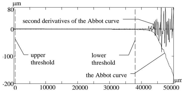
Figure 3: Detection of the lower and upper thresholds in the Abbot curve, oak sanded with P1000.
