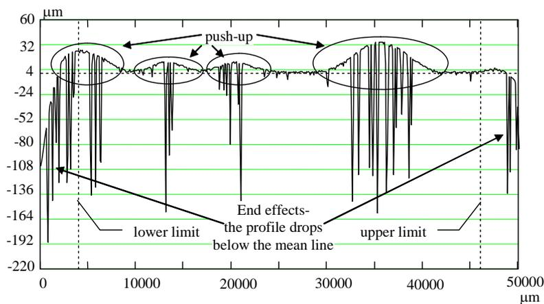
Figure 1: Roughness profile with "push-up" distortions and "end effects" introduced by the Gaussian filter in ISO 11652 1996, from oak sanded with P 1000. Vertical dashed lines mark the levels of the first and last half cut-off length of the filter.
