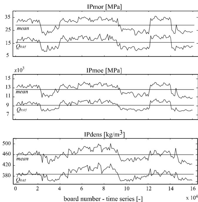
**Figure 1:** Time series of characteristic mean and 0.05-fractile values of all  $k=160$  sub-samples for IPmor, IPmoe and IPdens.
