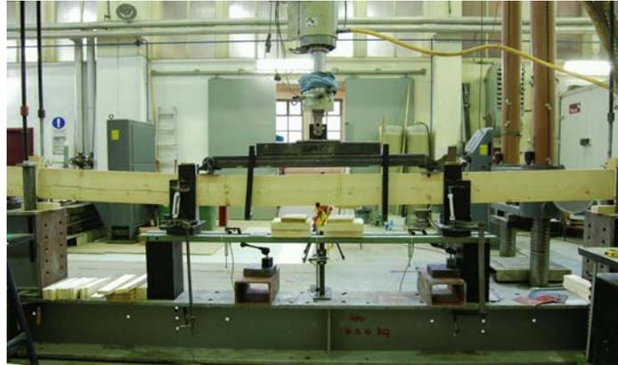
Figure 4: Destructive tests of boards 44 x 210 mm with lateral restraints
