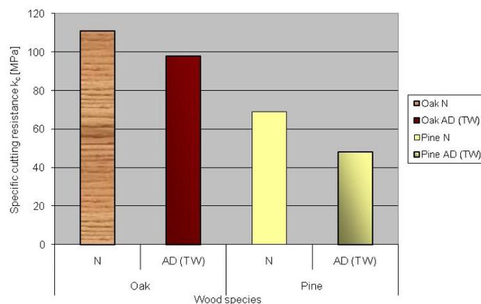
Figure 4: Comparison of specific cutting resistance of pine and oak for both methods of drying: natural (N) and accelerated (AD) in the kiln (values are valid for feed per tooth equal to  $f_z = 0.2$  mm)
