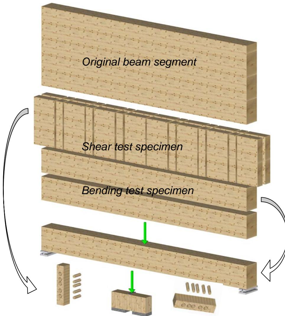
Figure 3: Test specimens cut from beam segments
