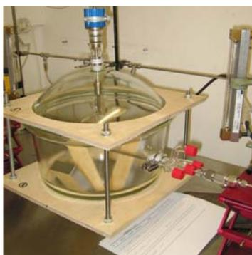
Figure 1: Emission test chamber
