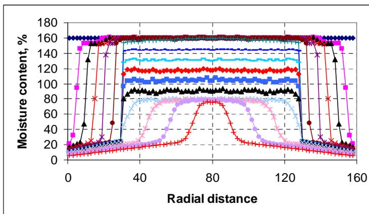
Figure 3: Moisture profiles assuming damaged surface layers.
