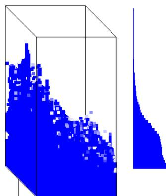
Figure 4: Calculated water absorption in an annual ring.
