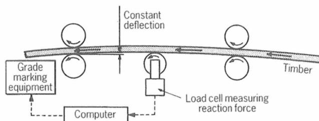
Figure 2: Schematic of Cook Bolinder strength grader.
