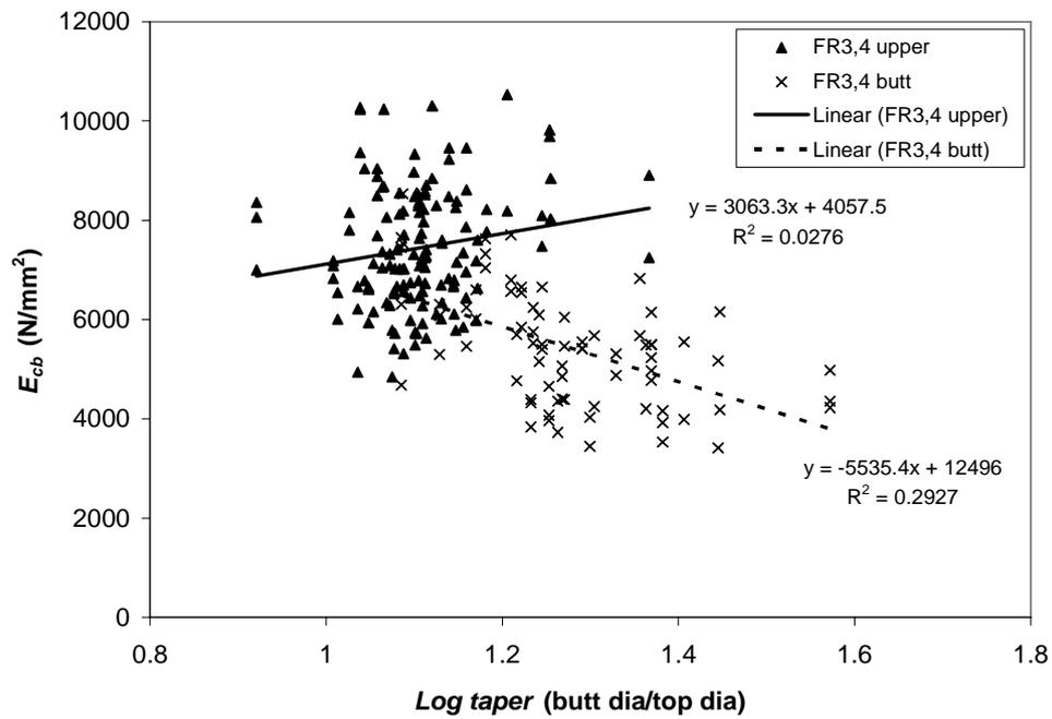
Figure 5:  $E_{cb}$  plotted against *Log taper* for groups of butt and upper logs.
