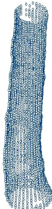
Figure 1: Log shape data obtained from industrial 3D laser scanner, from which variables such as *Log taper* were obtained.
