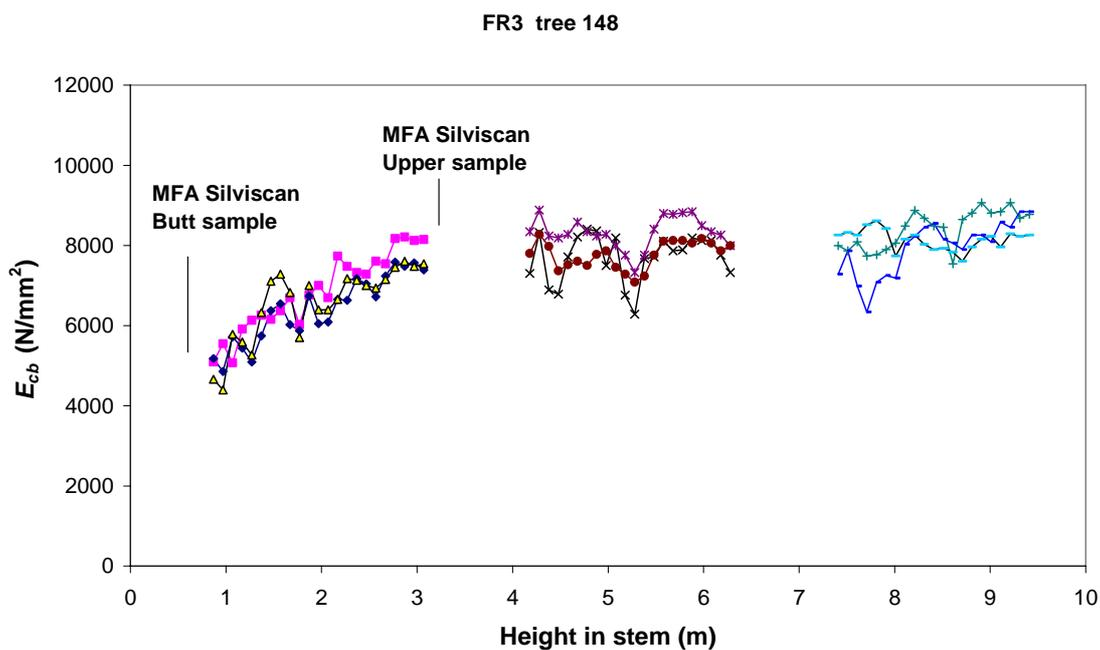
Figure 3:  $E_{cb}$  data plotted against height in stem, with position of MFA measurements shown.
