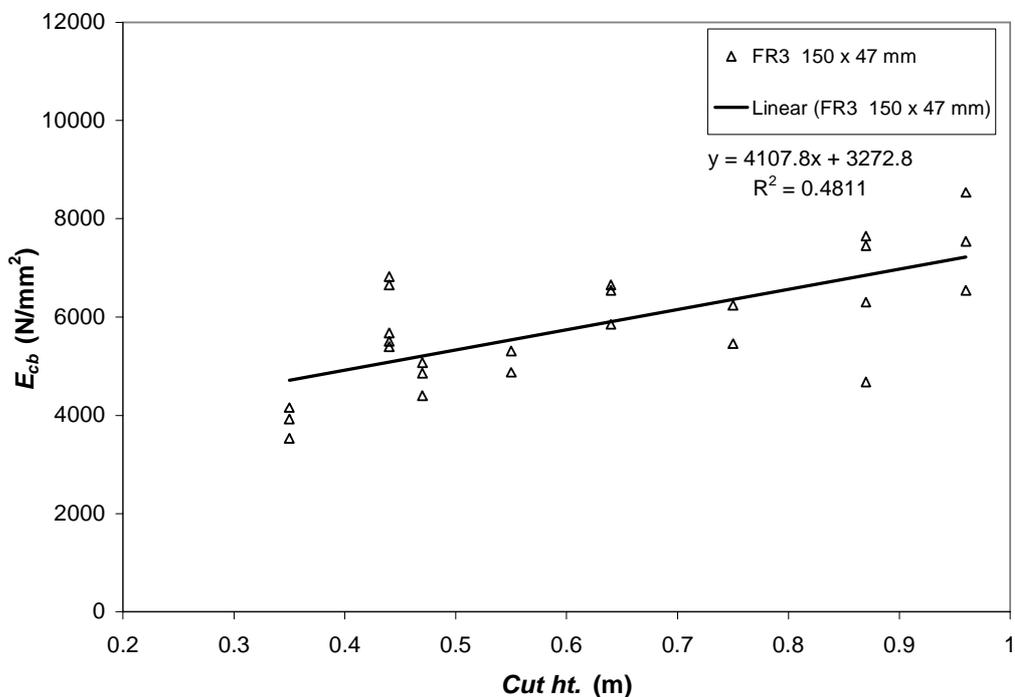
Figure 4:  $E_{cb}$  plotted against axial position *i.e.* Cut ht. (FR3 150 x 47 mm butt logs).
