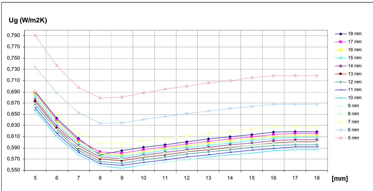
Figure 4. – Change of the  $U$ -value of triple glazing with Krypton fill as a function of the gap size (horizontal axis: outer gap size; the individual curves correspond to the different inner gap sizes)
