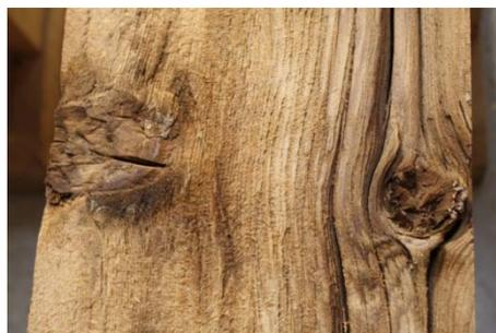
Figure 2: Weathered surface of an aged board
