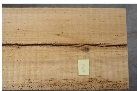
Figure 3: Damage due to insect attack
