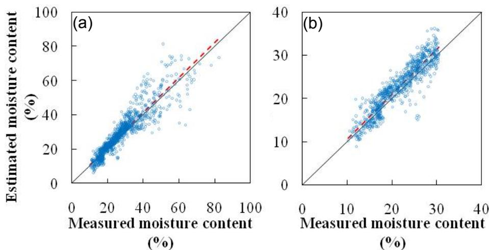
Figure 1: Measured vs. NIR estimated moisture for wide range of moisture (a) and hygroscopic range of moisture (b) with line 1000 mm/s. The dotted line is the regression - solid line R<sup>2</sup>=1.
