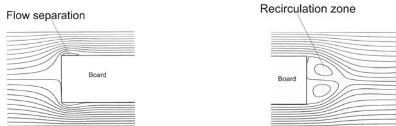
a – The leading edge of the first board b – The trailing edge of the last board Figure 1: The stream lines contour of the current variant (Sun 2001)
