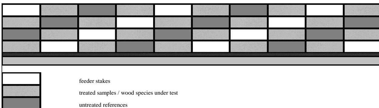
Figure 1: Positioning of specimens in a block
