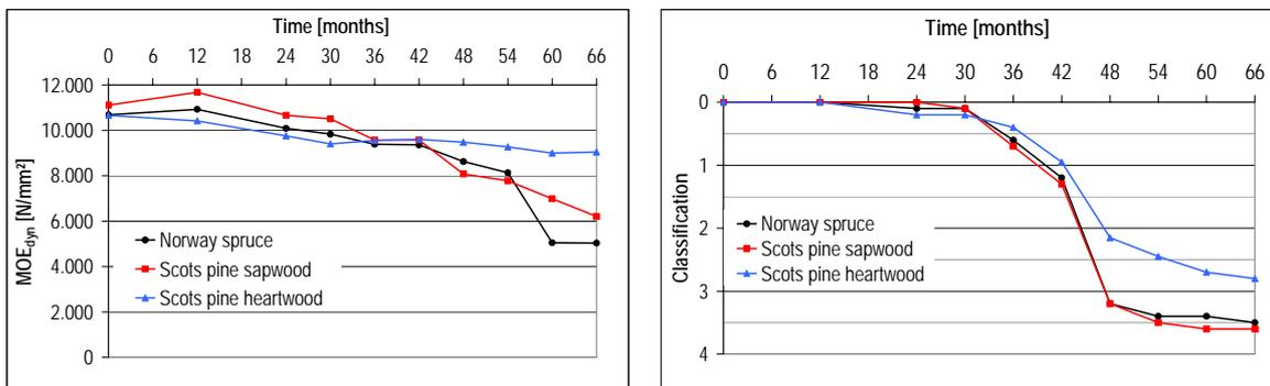
Figure 4: Evaluation of MOE<sub>dyn</sub> (left) and pick-test (right), mean values of B1
