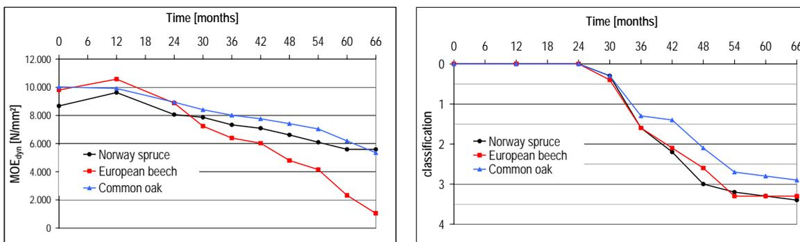
Figure 5: Evaluation MOE<sub>dyn</sub> (left) and pick-test (right), mean values of B2
