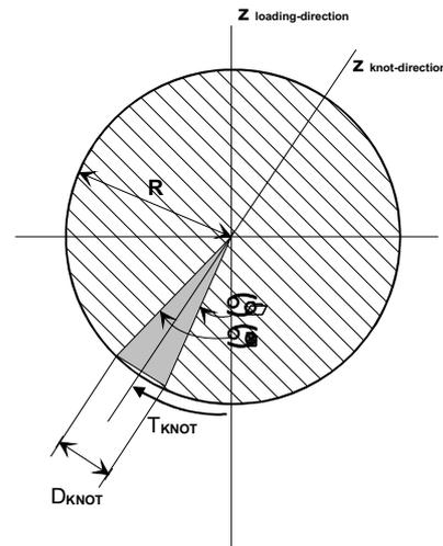
**Figure 4: Knot position projected at the cross-section area**
