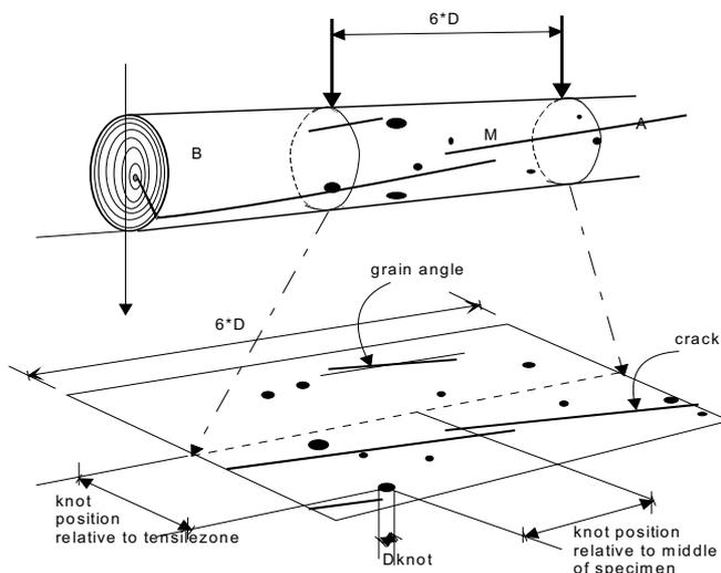
**Figure 2: Projection of the knots, slope of grain and fissures on the transparent paper**
