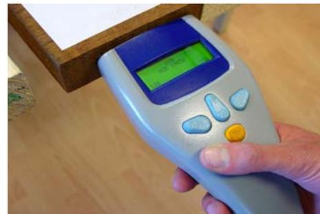
Figure 7: Timber Grader MTG
