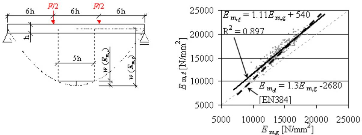
**Figure 3: Measuring principle and correlated results for local ( $E_{m,\ell}$ ) and global ( $E_{m,g}$ ) bending MOE of all three TMTB samples**
