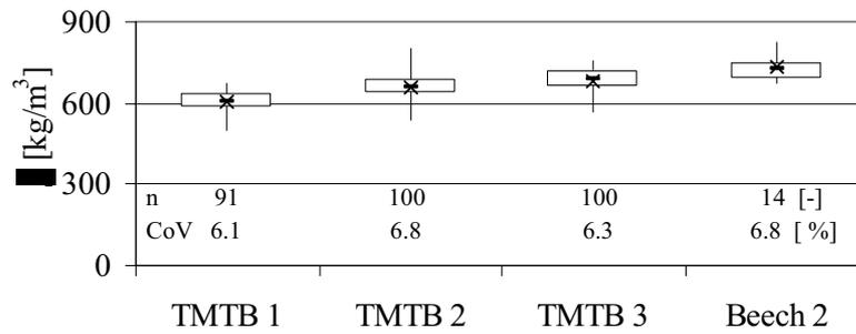
**Figure 1: Density of three TMTB samples and an untreated beech sample. The mean moisture content of the TMTB samples varied between 5.5% and 6.5%, in the untreated beech sample the mean moisture added up to 13.2%**
