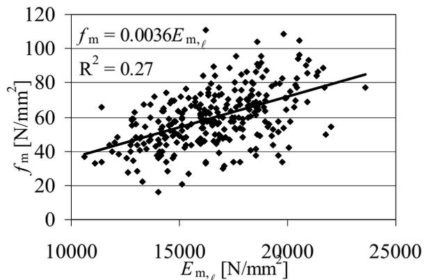
**Figure 6: Matrix of coefficients of correlation  $R^2$  of several possible parameters to grade TMTB and a graph showing the linear correlation of measured local MOE  $E_{m,\ell}$  and bending strength  $f_m$  as an example**
