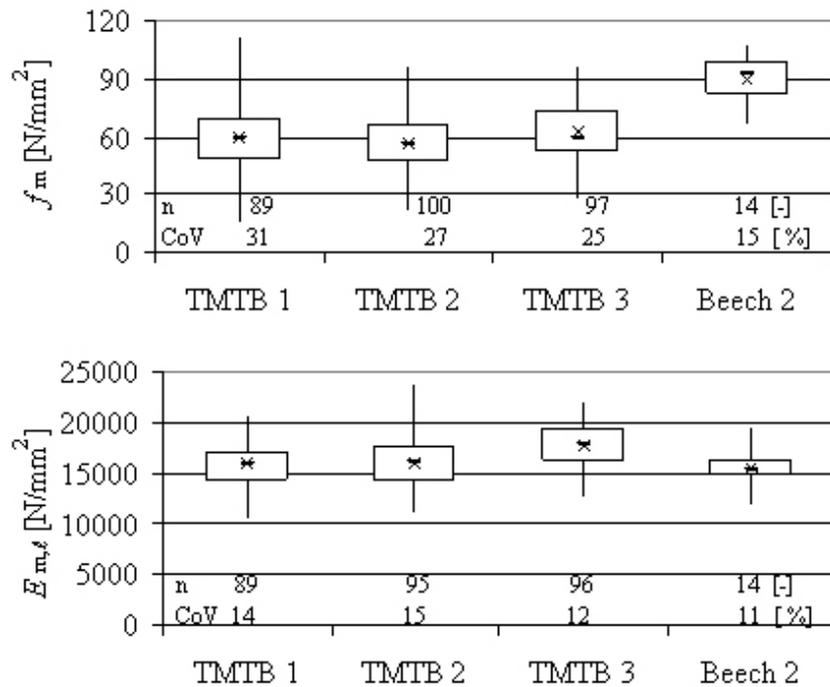
**Figure 2: Bending strength  $f_m$  and bending MOE  $E_{m,l}$  of three TMTB sample and one untreated beech sample**
