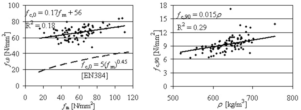
**Figure 5: Compression strength parallel to grain  $f_{c,0}$  in relation to bending strength  $f_m$  (left) and compression strength perpendicular to grain  $f_{c,90}$  versus density  $\rho$  (right)**
