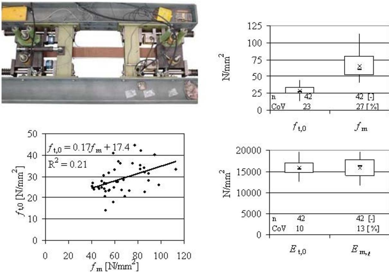
**Figure 4: Tension strength  $f_{t,0}$  and tension MOE  $E_{t,0}$  parallel to the grain compared to (flatwise) bending strength  $f_m$  and MOE  $E_{m,t}$  of one TMTB sample consisting of  $n = 42$  boards**
