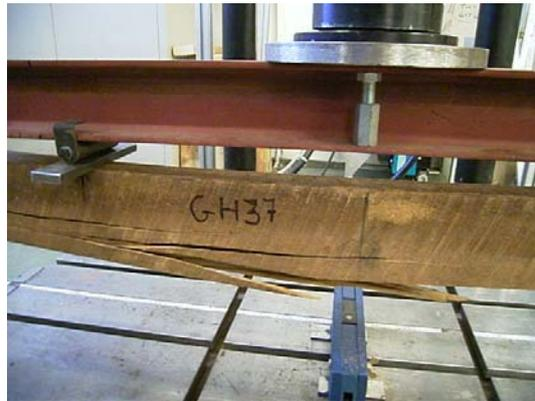
**Figure 6: Typical failure of a tropical hardwood beam in a bending test**
