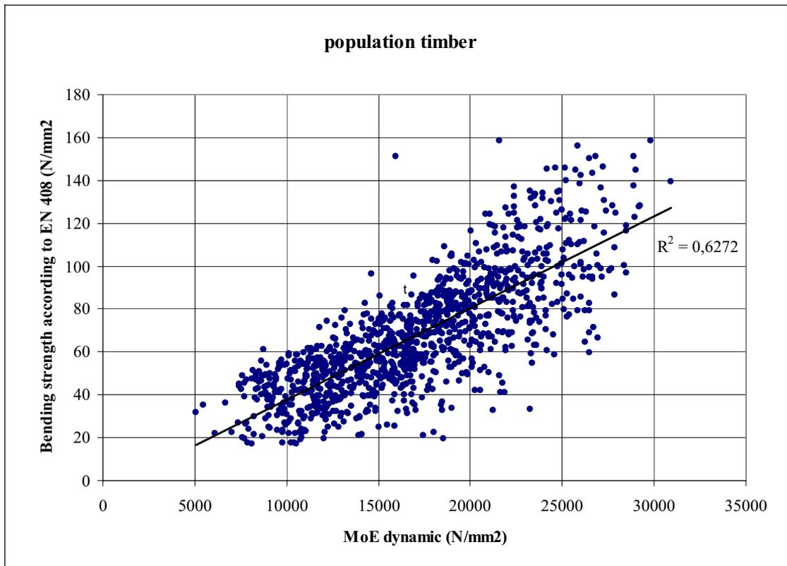
**Figure 7: Relationship between non-destructive measurements and the bending strength with combined test results of a number of species**
