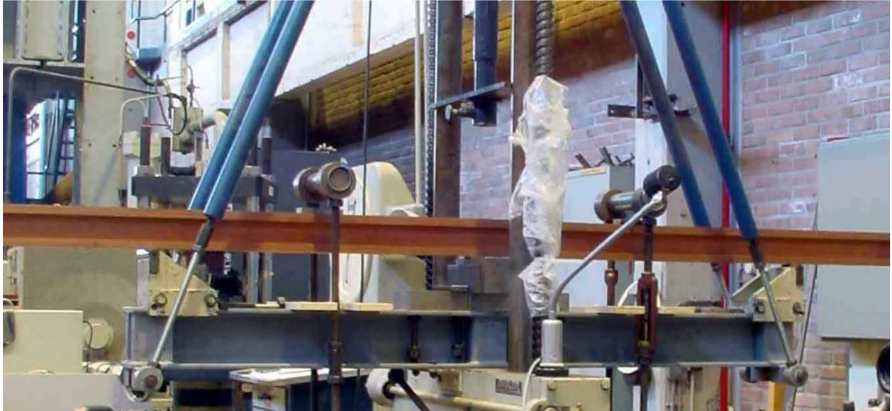
*Figure 8: Test set-up I-beams for determination of the shear strength*
