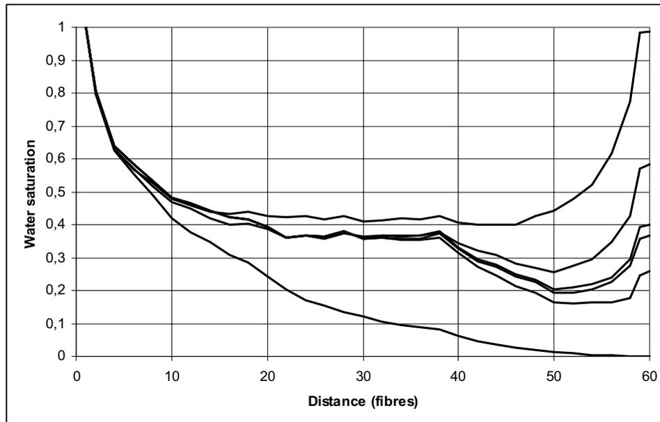
**Figure 4:** *Calculated moisture profiles in the vertical direction for different rates of evaporation from the upper surface. The uppermost curve represents a very low evaporation rate and the lowest curve a very high (infinite) rate*
