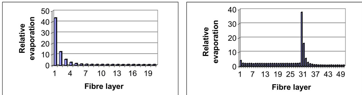
**Figure 2: Location of the evaporation front calculated with a capillary fibre network model. To the left the result for an undamaged sample is given and to the right with a 30 fibre thick damaged layer with increasing structure openness towards the surface**
